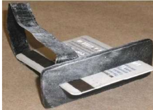
Figure 1 Lebanese loop fraud – special additional equipment - example
