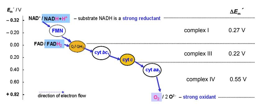
The standard electrode potential difference  $\Delta E^{\circ}$  for the reduction of O<sub>2</sub> with NADH **1.14 V** drives the electron transport through the chain. The corresponding standard free energy  $\Delta G^{\circ} = -220 \text{ kJ mol}^{-1}$ .
