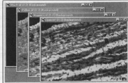
Figure 2: Scanned picture decomposed by the morphometric software into 3 colour (cyan, magenta, yellow) and one black-white component
