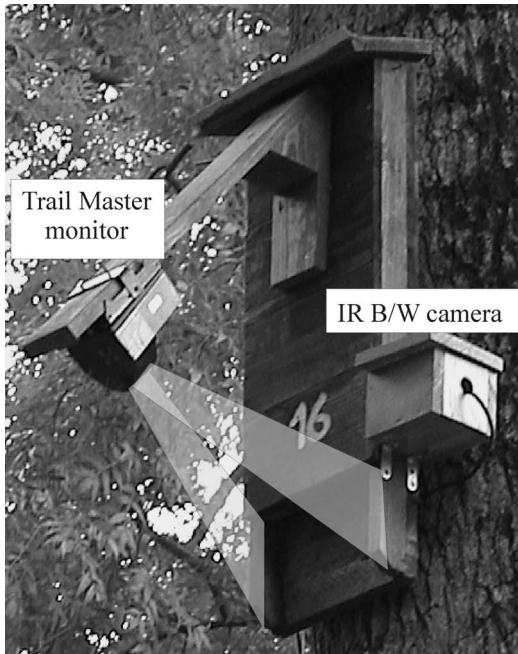
FIG. 1. Wooden bat box. Monochrome (B/W) IR diode camera monitored the entrance of the box and was connected to a battery and digital recorder on the ground. Two grey shapes mark out a space monitored by passive IR Trail Master monitor (TM550) on a bracket in front of the bat box. Internal temperature was measured with help of Hobo Data Loggers (Onset Computer Corporation) (inside box). Sensor measuring external temperature was placed outside roughly half a meter from the bat box
