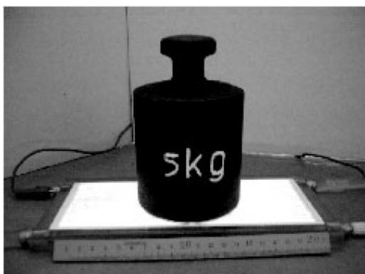
Fig. 3 Cooled 500 W plasma panel constructed on the base of coplanar diffuse surface barrier discharge. The picture illustrates mechanical and “electrical” robustness of the panel.
