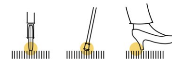
a) Gratings with small mesh size allowing unhindered movement of wheels, walking sticks and shoe heels
