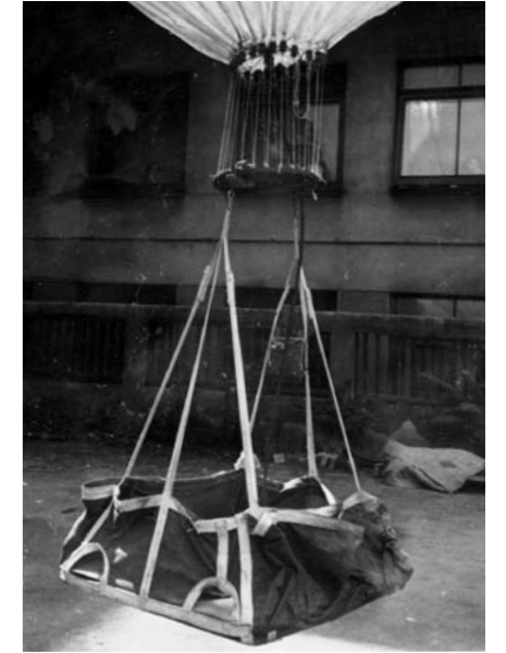
▲ The folding basket of the "invisible" balloon, in which Blažek and Jakoubě crashed.
