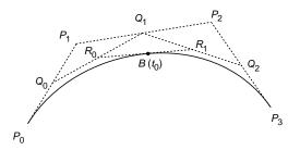
Suppose the points we have selected are  $P_0(x_0, y_0), \ldots, P_3(x_3, y_3)$ . The deCastlejau algorithm for finding the point on the curve that corresponds to the parameter value  $t = t_0, 0 \le t_0 \le 1$ , is based on linear interpolation, and, indeed, applying it repeatedly: A parametrization of the segment  $P_0P_1$  is given by
