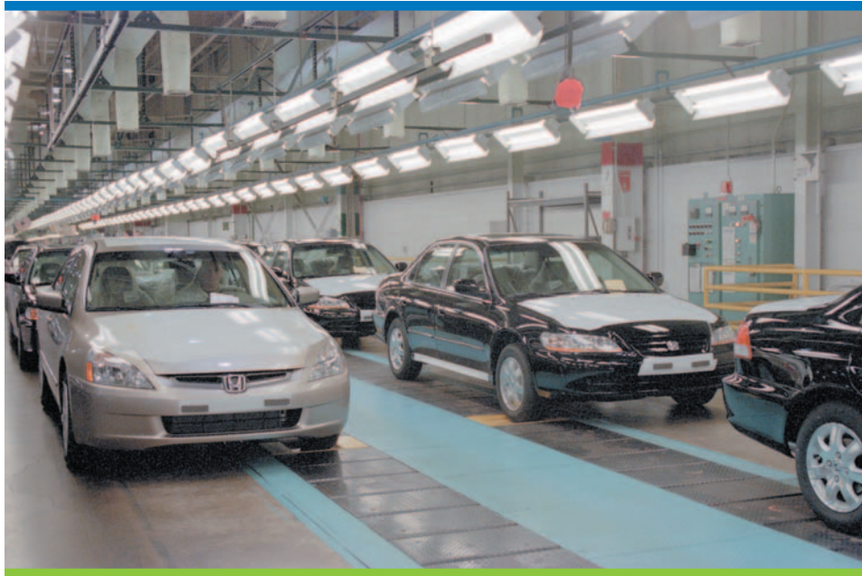
THIS HONDA ASSEMBLY LINE ALLOWS TECHNICIANS THE FLEXIBILITY TO TRADE WORK ELEMENTS, AND ALLOWS MANAGEMENT TO ADD OR SUBTRACT OPERATORS AS NECESSARY.
