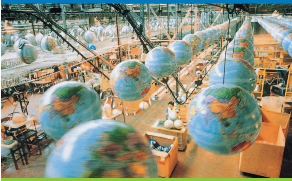
PLANET EARTH ORBITING THE ASSEMBLY LINE IN A GLOBE FACTORY. THE GLOBES ARE MOVING THROUGH THE FACTORY USING A TRANSPORT SYSTEM SUSPENDED FROM THE CEILING OF THE FACTORY.
