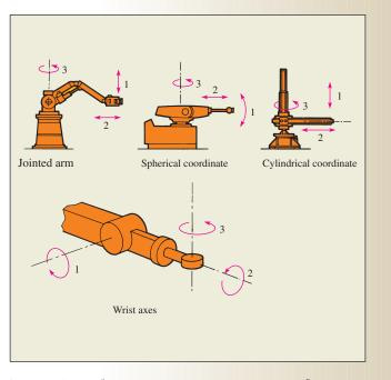
SC.3—Typical Robot Axes of Motion
