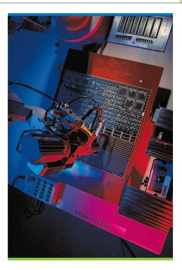
some models can be "taught" a sequence of motions in a three-dimensional pattern. As a worker moves the end of the robot arm through the required motions, the robot records this pattern in its memory and repeats it on command. As shown in the box "Formula for Evaluating a Robot Investment," robots are often justified based on labor savings.
