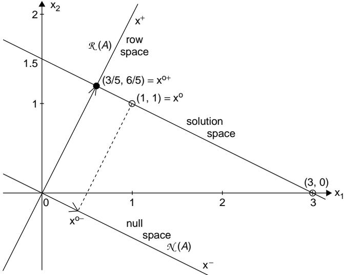
**Figure 2.1** A minimum-norm solution.
