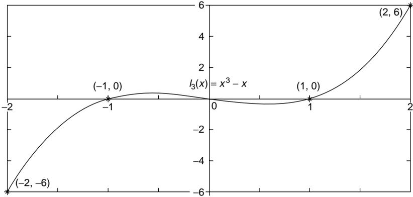
Figure 3.1 The graph of a third-degree Lagrange polynomial.
