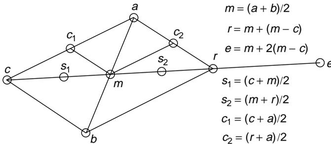
**Figure 7.3** Notation used in the Nelder–Mead method.
