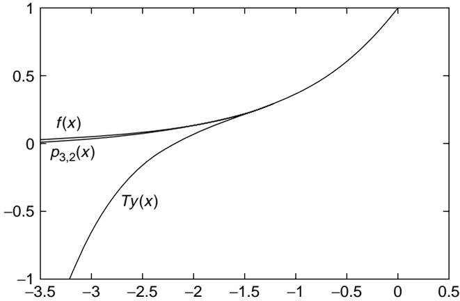
**Figure 3.6** Padé approximation and Taylor series expansion for  $f(x) = e^x$  (Example 3.2).
