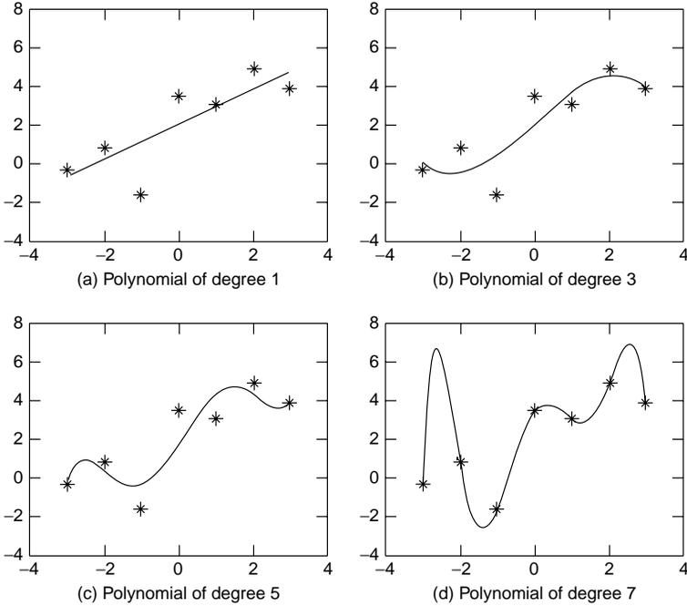
**Figure 3.10** Polynomial curve fitting by the LS (Least-Squares) method.
