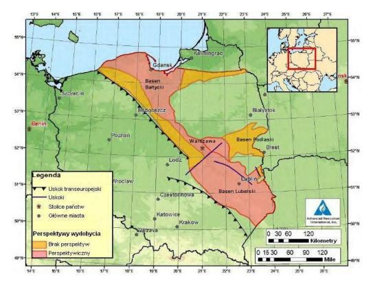
Forecasts indicate that the potential of shale gas deposits are located at depths from 1200-2500 m in the northern part of the lane to 2500-4500 m in the south part. There is estimated that the cost of a vertical drilling, depending on the depth, could range from 6 to 13 million dollars.
