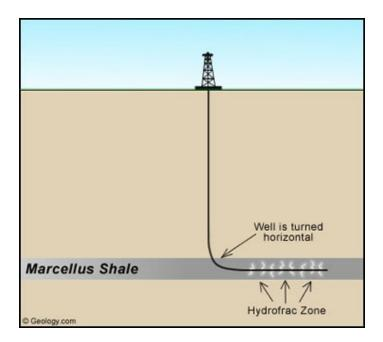
Hydraulic fracturing involves pumping into a selected section of the drilling hole fluid under high pressure, consisting of a carrier (mainly water) with additional filler materials (mainly sand of selected grain and mechanical strength) and extra chemicals (mainly in order to enhance viscosity). The liquid under pressure creates a cracks in the rock structure, while sand fills and maintains the gap, creating a new way for gas migration in the hole.
