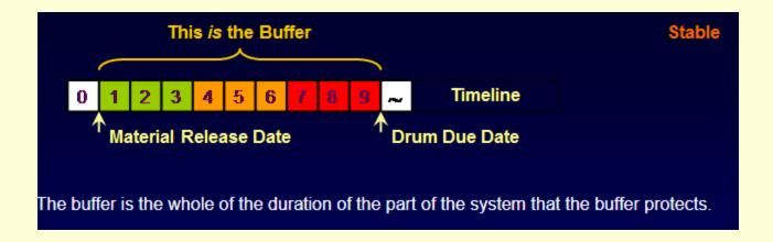
The order of priority for processing parts assigned to different Work Orders is determined by colour (as in traffic lights)
