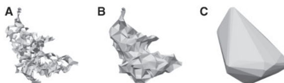
Fig. 2. Alpha shape model obtained with different alpha values. (A) The molecular surface cannot be obtained completely if the alpha value is too small. (B) Surface obtained perfectly with a proper alpha value. (C) The surface will lose some details if the alpha value is too large.
