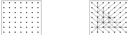
Fig. 2. Discretization of the state space. The larger bullets represent precomputed configurations (compare with the figure 1). On the left only configurations in the grid points are depicted, whereas on the right, also intermediate states are included (represented by smaller bullets).
