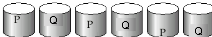
(g) RAID 6: P + Q redundancy
