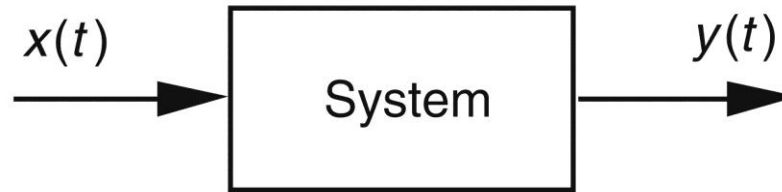
Figure 6-5 System described by Eq. (6-6). The system's input and output are the continuous-time functions x(t) and y(t) respectively.
