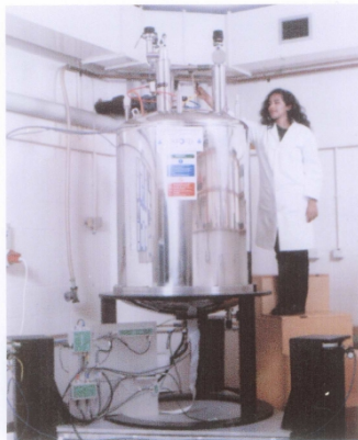
The superconducting magnet of a 600 MHz NMR Spectrometer
