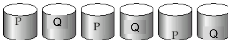
(g) RAID 6: P + Q redundancy
