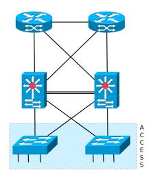
▶ access layer – connects network end devices to computer network (clients and servers). Access layer switches are placed on premises, where it meets physical topology constraints (100m distance from clients Cat 5E cables)
