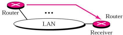
Case 3. A router receives a packet to be sent to a host on another network. It must first be delivered to the appropriate router.
