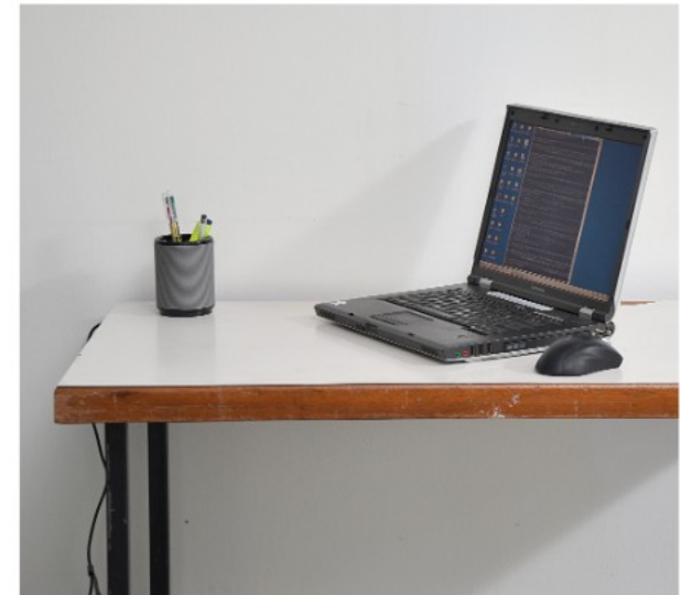
(b) Target (Lenovo 3000 N200), performing ECDH decryption operations, on the other side of the wall.
