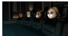
Oculus Social Alpha, which was an application for Samsung Gear VR. Multiple users could meet in a virtual world and socialize. In this case, they are watching a movie together in a theater. Their head movements are provided using head tracking data. They are also able to talk to each other with localized audio
