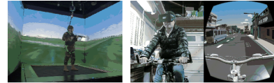
(a) An omnidirectional treadmill used in a CAVE system by the US Army for training. (b) A home-brew bicycle riding system connected to a VR headset, developed by Paul Dyan
