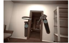
A virtual "laser pointer" that follows a parabolic arc so that a destination for teleportation can be easily specified as a point on the floor. (Image from the Budget Cuts game on the HTC Vive platform.)
