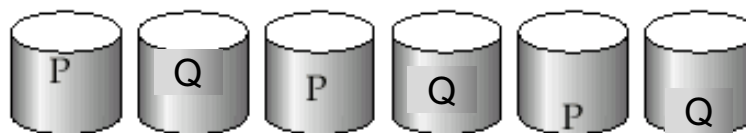
(g) RAID 6: P + Q redundancy
