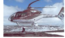
The wings of a flying helicopter are apparently bent backwards due to the rolling shutter effect
