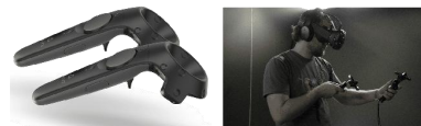
(a) A pair of hand-held controllers that came with the HTC Vive headset in 2016; the device includes side buttons, a trigger, and a touch pad for the thumb. (b) A user trying the controllers (prototype version)
