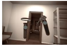
A virtual "laser pointer" that follows a parabolic arc so that a destination for teleportation can be easily specified as a point on the floor. (image from the Budget Cuts game on the HTC Vive platform.)
