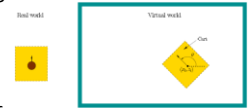
Locomotion along a horizontal terrain can be modeled as steering a cart through the virtual world. A top-down view is shown. The yellow region is the matched zone, in which the user's viewpoint is tracked. The values of x_c , z_c , and \theta are changed by using a controller
