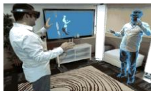
Holographic communication research from Microsoft in 2016. A 3D representation of a person is extracted in real time and superimposed in the world, as seen through augmented reality glasses (HoloLens)
