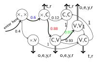
$\begin{array}{l} p(t|C) = .3 \\ p(r|C) = .7 \\ p(o|V) = .1 \\ p(e|V) = .3 \\ p(y|V) = .4 \\ p(r|V) = .2 \end{array}$
