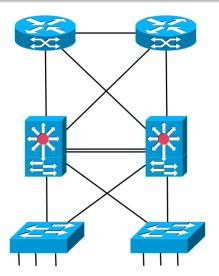
Core layer: backbone, connection to the "outside world" – fast, reliable, efficient
