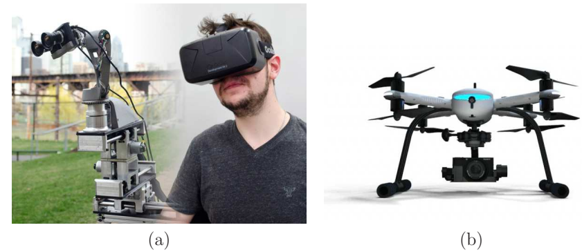
Figure 1.11: Examples of robotic avatars: (a) The DORA robot from the University of Pennsylvania mimics the user's head motions, allowing him to look around in a remote world while maintaining a stereo view (panoramas are monoscopic). (b) The Plexidrone, a low-cost flying robot that is designed for streaming panoramic video.
