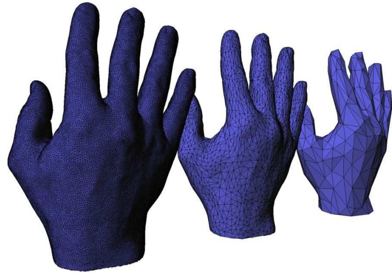
Figure 7.16: A variety of mesh simplification algorithms can be used to reduce the model complexity while retaining the most important structures. Shown here is a simplification of a hand model made by the open-source library CGAL. (Figure by Fernando Cacciola.)
