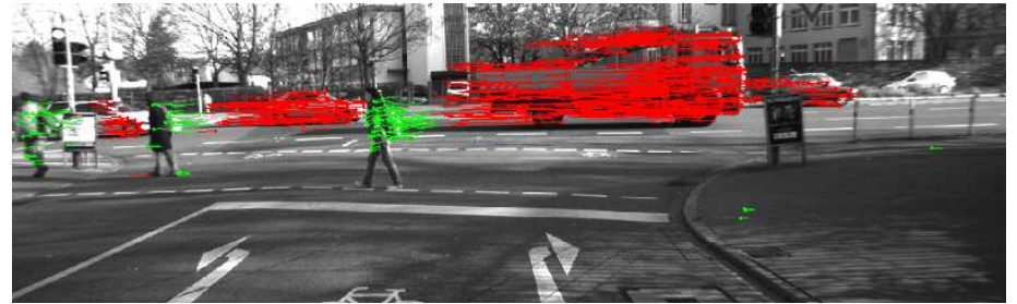
Figure 8.13: The optical flow of features in an image due to motion in the world. These were computed automatically using image processing algorithms. (Image by Andreas Geiger, from Max Planck Institute for Intelligent Systems in Tübingen.)
