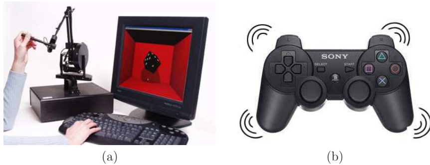
Figure 2.8: Two examples of haptic feedback devices. (a) The Geomagic Phantom allows the user to feel strong resistance when poking into a virtual object with a real stylus. A robot arm provides the appropriate forces. (b) Some game controllers occasionally vibrate.
