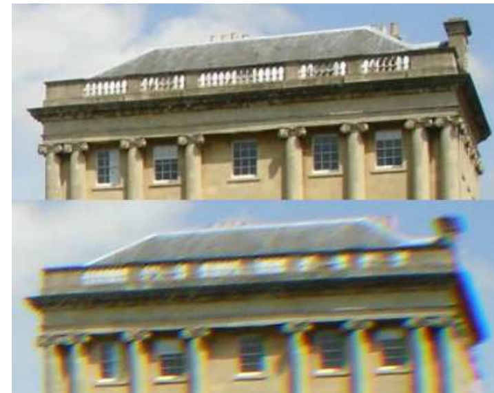
Figure 4.18: The upper image is properly focused whereas the lower image suffers from chromatic aberration. (Figure by Stan Zurek.)
