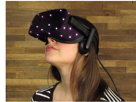
Figure 9.13: The Oculus Rift headset contains IR LEDs hidden behind IR-transparent plastic. (Photo by iFixit.)
