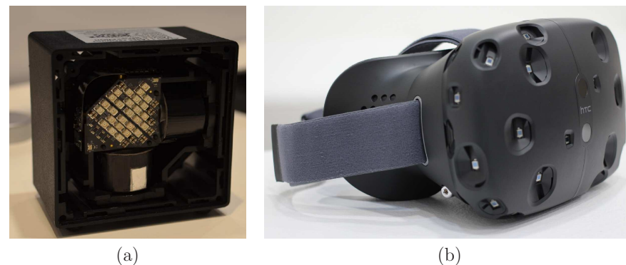
Figure 9.16: The laser-based tracking approach used in the HTC Vive headset: (a) A base station contains spinning drums that emit horizontal and vertical sheets of IR light. An array of IR LEDs appears in the upper left, which provide a synchronization flash. (b) Photodiodes in pockets on the front of the headset detect the incident IR light.
