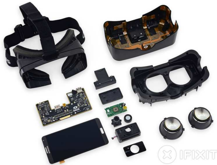
Figure 2.12: Disassembly of the Oculus Rift DK2 headset (image by ifixit).
