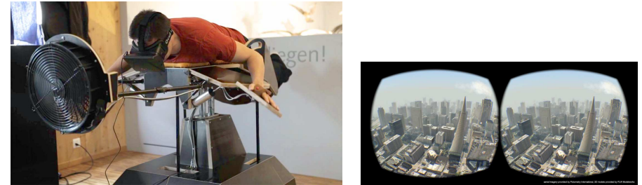
Figure 1.1: In the Birdly experience from the Zurich University of the Arts, the user, wearing a VR headset, flaps his wings while flying over virtual San Francisco. A motion platform and fan provide additional sensory stimulation. The figure on the right shows the stimulus presented to each eye.
