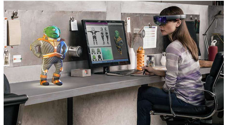
Figure 1.19: The Microsoft HoloLens uses advanced see-through display technology to superimpose graphical images onto the ordinary physical world, as perceived by looking through the glasses.
