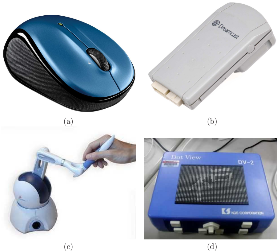
Figure 13.4: (a) The Logitech M325 wireless mouse with a scroll wheel that provides tactile feedback in the form of 72 bumps as the wheel performs a full revolution. (b) The Sega Dreamcast Jump Pack (1999), which attaches to a game controller and provides vibrations during game play. (c) Haptic Omni pen-guiding haptic device, which communicates pressure and vibrations through the pen to the fingers. (d) The KGS Dot View Model DV-2, which is a haptic pin array. The pins are forced upward to simulate various textures as the finger tip scans across its surface.
