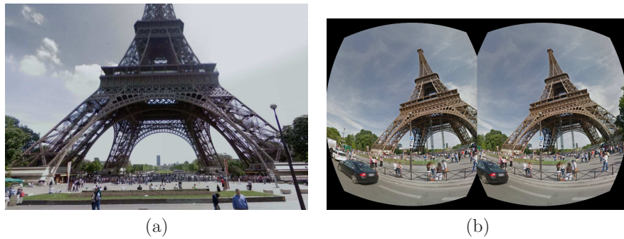
Figure 1.9: A simple VR experience that presents Google Street View images through a VR headset: (a) A familiar scene in Paris. (b) Left and right eye views are created inside the headset, while also taking into account the user's looking direction.
