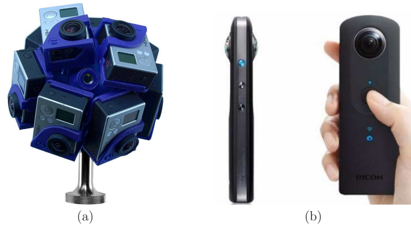
Figure 7.23: (a) The 360Herros Pro10 HD is a rig that mounts ten GoPro cameras in opposing directions to capture panoramic images. (b) The Ricoh Theta S captures panoramic photos and videos using only two cameras, each with a lens that provides a field of view larger than 180 degrees.
