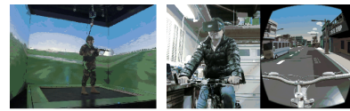
(a) An omnidirectional treadmill used in a CAVE system by the US Army for training. (b) A home-brew bicycle riding system connected to a VR headset, developed by Paul Ryan.
