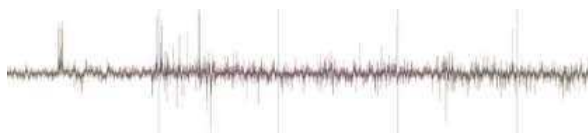
Figure 4: Difference between averages of AES power traces sorted on input bit 18 vertically magnified by a factor of 25. The spikes show the influence of bit 18 on the power consumption of the device.
