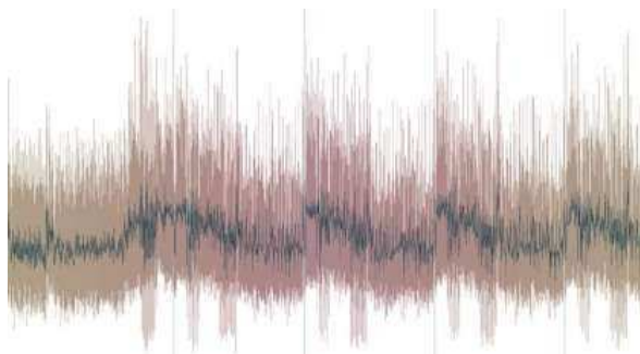
Figure 3: Power trace of device performing a single AES encryption.
