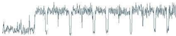
Figure 12: Data collected from HTC Evo 4G phone using near field antenna placed behind phone
