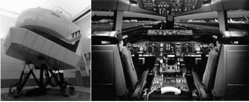
Advanced flight simulator of Boeing 777: (left) outside view, (right) inside view
