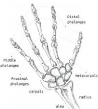
Top view of simplified human hand kinematic model (22 DOFs)
