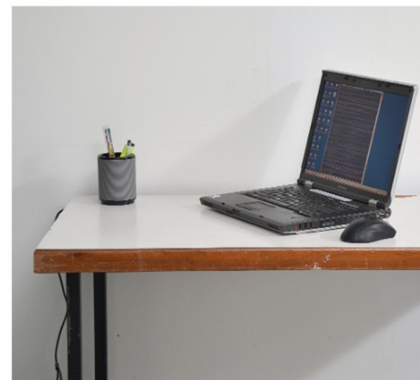
(b) Target (Lenovo 3000 N200), performing ECDH decryption operations, on the other side of the wall.
