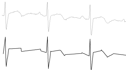
Figure 1.13. An example of a time series segmentation with its piecewise linear representation
