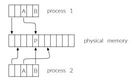
The address B may or may not be a valid address in the first process, and the same holds for A in the second process.
