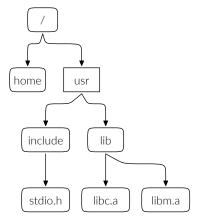
Usually, file systems are mounted onto empty directories: if /usr was not empty on the left (root) file system, its content would be hidden by the mount.
