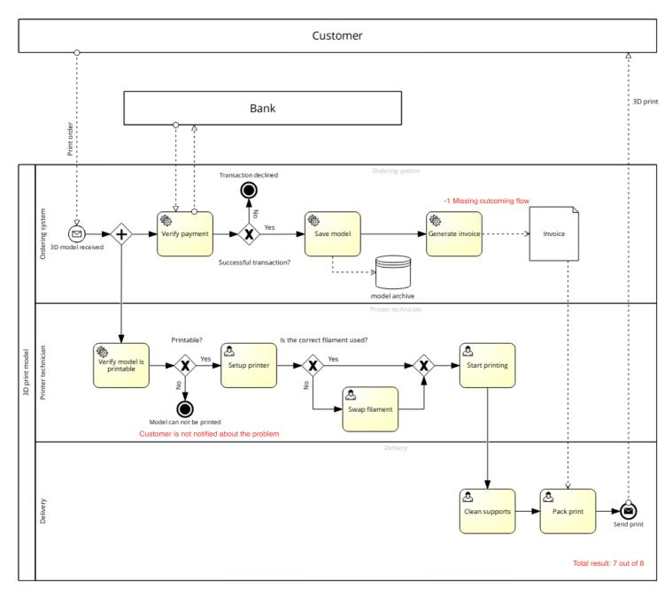
Customer wants to print 3D file on a 3D printer. He creates order, which is verified both payment wise and printability wise. If it is OK, technican sets up the printer, prints the file and delivery boy cleans the print, packs it and delivers it.
