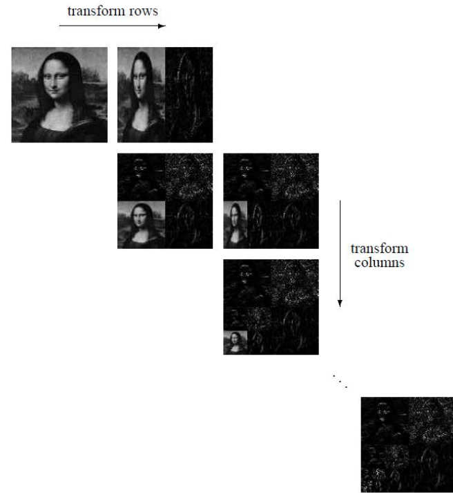
Figure 6 Nonstandard decomposition of an image. An example from Wavelets for Computer Graphics: A Primer [1]
