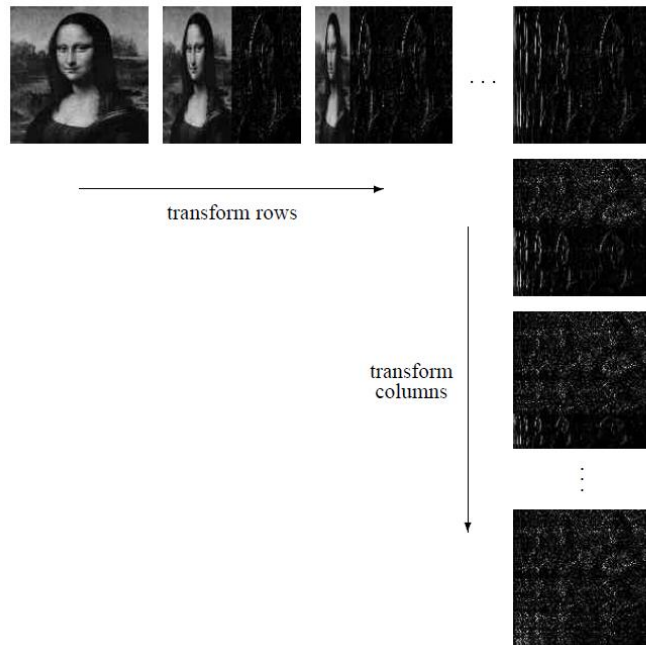
Figure 5 Standard decomposition of an image. An example from Wavelets for Computer Graphics: A Primer [1]
