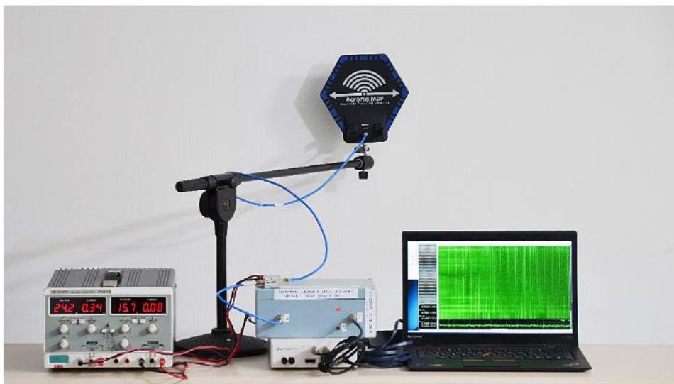
(a) Attacker's setup for capturing EM emanations. Left to right: power supply, antenna on a stand, amplifiers, software defined radio (white box), analysis computer.
