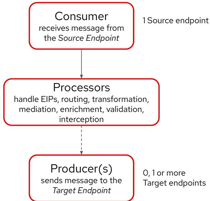
**Camel route** describes the step-by-step movement of a Message from a source endpoint, through arbitrary types of decision-making routines (such as filters and routers) to a destination endpoint (if any)
