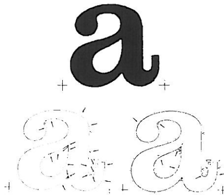
Fig. 8. Above: Possible input for digitizing. Left: An auto-traced character has to be fine-tuned. Right: A hand-digitized characters leaves less points for fine-tuning of the outline.
