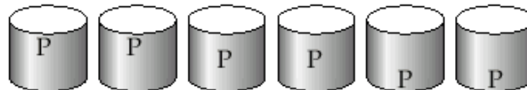
(g) RAID 6: P + Q redundancy
