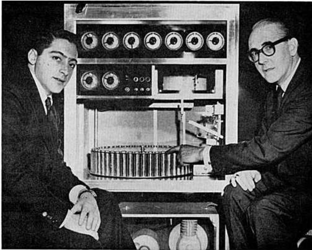
THE BRAINS OF SMELL-O-VISION—Michael Todd, Jr. (left) sits beside master control and scent energizer of the Smell-O-Vision system with its inventor Hans Lube. Latter points to the multitude of vials each containing a different scent which is selectively projected through tubes to every seat in theatre on signal triggered from picture's sound track.
