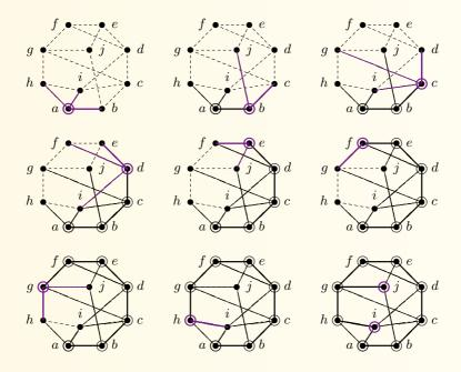
Various networking applications are often demanding not only that a graph is connected, but that it will stay connected even after failure of some small number of nodes (vertices) or links (edges).
