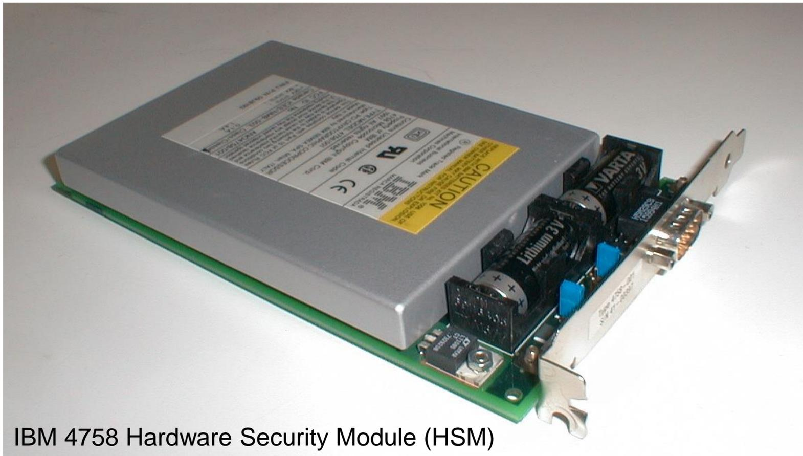
IBM 4758 Hardware Security Module (HSM)
