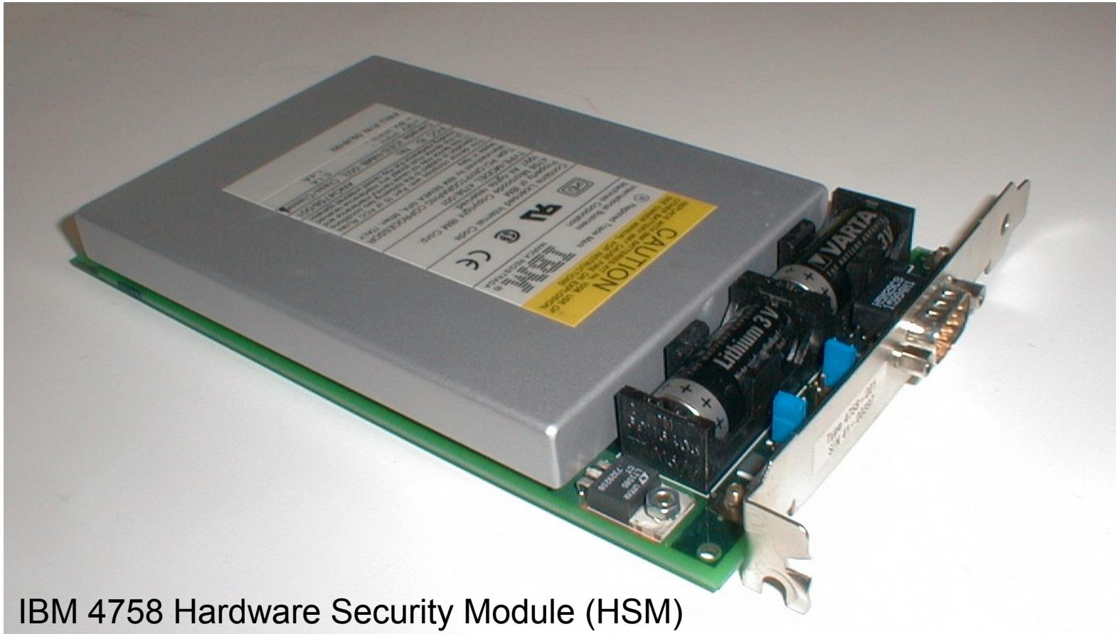
IBM 4758 Hardware Security Module (HSM)
