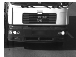
(b) Vehicle damages (e.g. missing letters)
