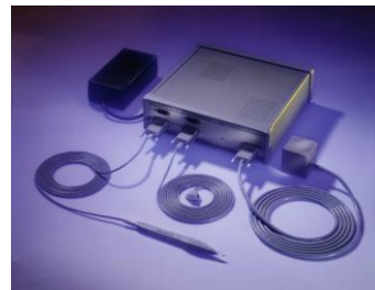
Polhemus FASTRACK electromagnetic tracker
