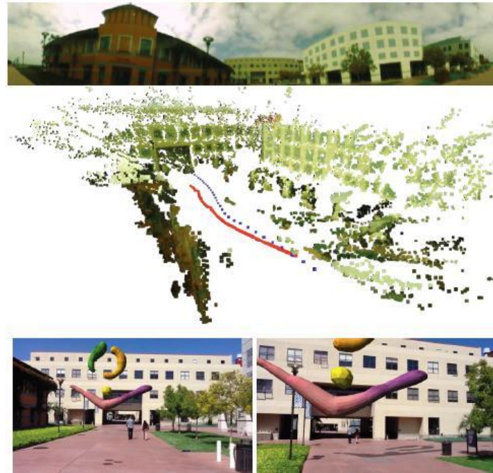
Figure 11.1: Wide area AR tracking using panorama imagery (top) processed into a point cloud dataset (middle) and used for AR localisation (bottom). [Ventura and Hollerer, 2012].
