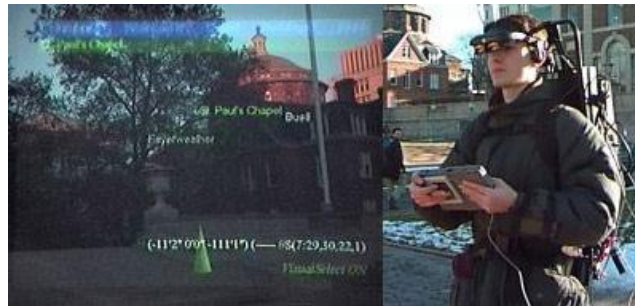
(a) Feiner's Touring Machine [Feiner et al., 1997]
