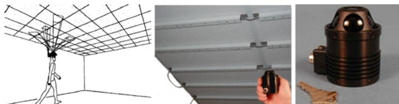
Figure 4.3: Conceptual drawing of inside-looking-out system (Left). Roof mounted infrared led arrays (Middle) and the Hi-ball camera tracker (Right). [Welch et al., 1999]
