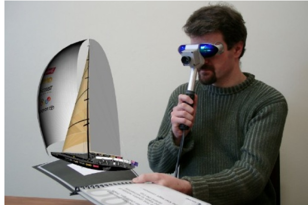
Figure 7.4: Tangible AR interface with a physical book with virtual object overlaid on it.
