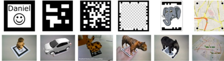
Figure 4.8: Markers supported by Studierstube ES: Template Markers, BCH Markers, DataMatrix Markers, Frame Markers, Split Markers, and Grid Markers. [Schmalstieg and Wagner, 2009]
