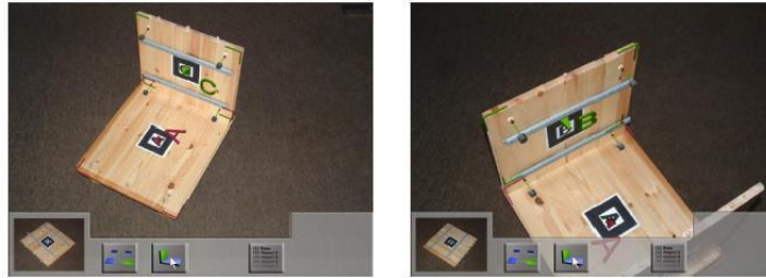
Figure 6.5: AR furniture assembly application created with the AMIRE framework. [Zauner et al., 2003]
