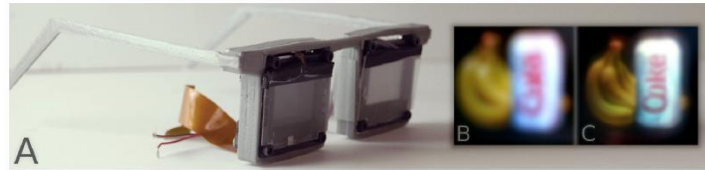
Figure 11.7: Computational AR eyeglasses and view through the display. [Maimone and Fuchs, 2013]
