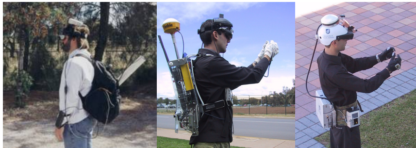
(b) Thomas and Piekarski's wearable AR systems in 1998, 2002, and 2006. http://www.tinmith.net/backpack.htm
