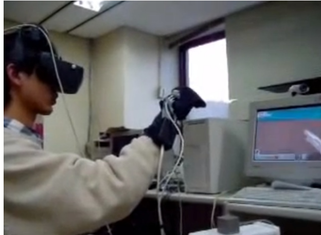
Figure 2.2: Typical Virtual Reality system with an immersive head mounted display, data glove, and tracking sensors. [Lee et al., 2002]
