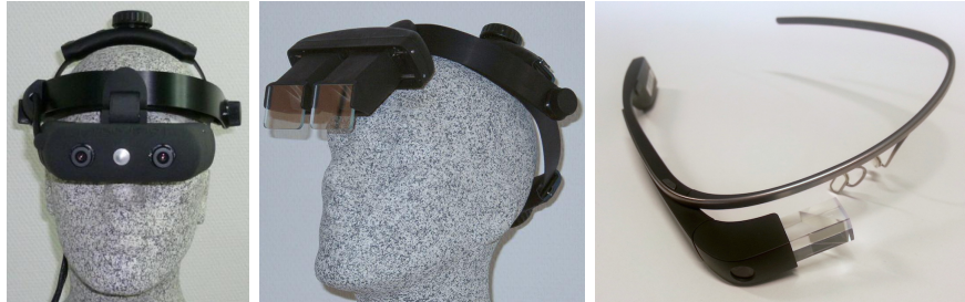
Figure 5.12: Various types of head-attached displays. From left to right: video and optical see-through HMD from Trivisio ( www.trivisio.com ), and Google Glass ( http://www.google.com/glass )
