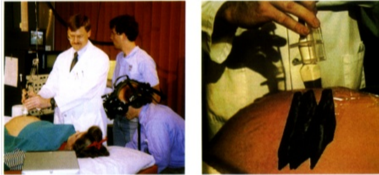
Figure 4.2: 2D slices of ultrasound data is overlaid on a patient's abdomen. Both the HMD and ultrasound transducer are tracked using a Polhemus magnetic tracker. [Bajura et al., 1992]
