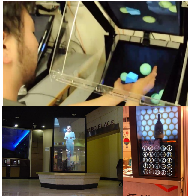
Figure 5.7: Optical see-through displays using half-mirror [Hilliges et al., 2012] (top), transparent projection film (lower left, http://www.laser-magic.com/transscreen.html ), and transparent LCD (lower right).
