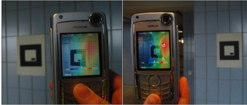
Figure 11.4: Using mobile AR for visualization ubiquitous computing sensor data. [Rauhala et al., 2006]
